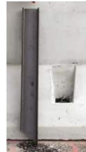
The road restraint device has also reached high performance levels with particular reference to the ASI index (equal to 1.26) whose reduction was possible using a new barrier geometry that, through three different planes having different inclinations, contributes to damping the kinetic energy following the impact.
